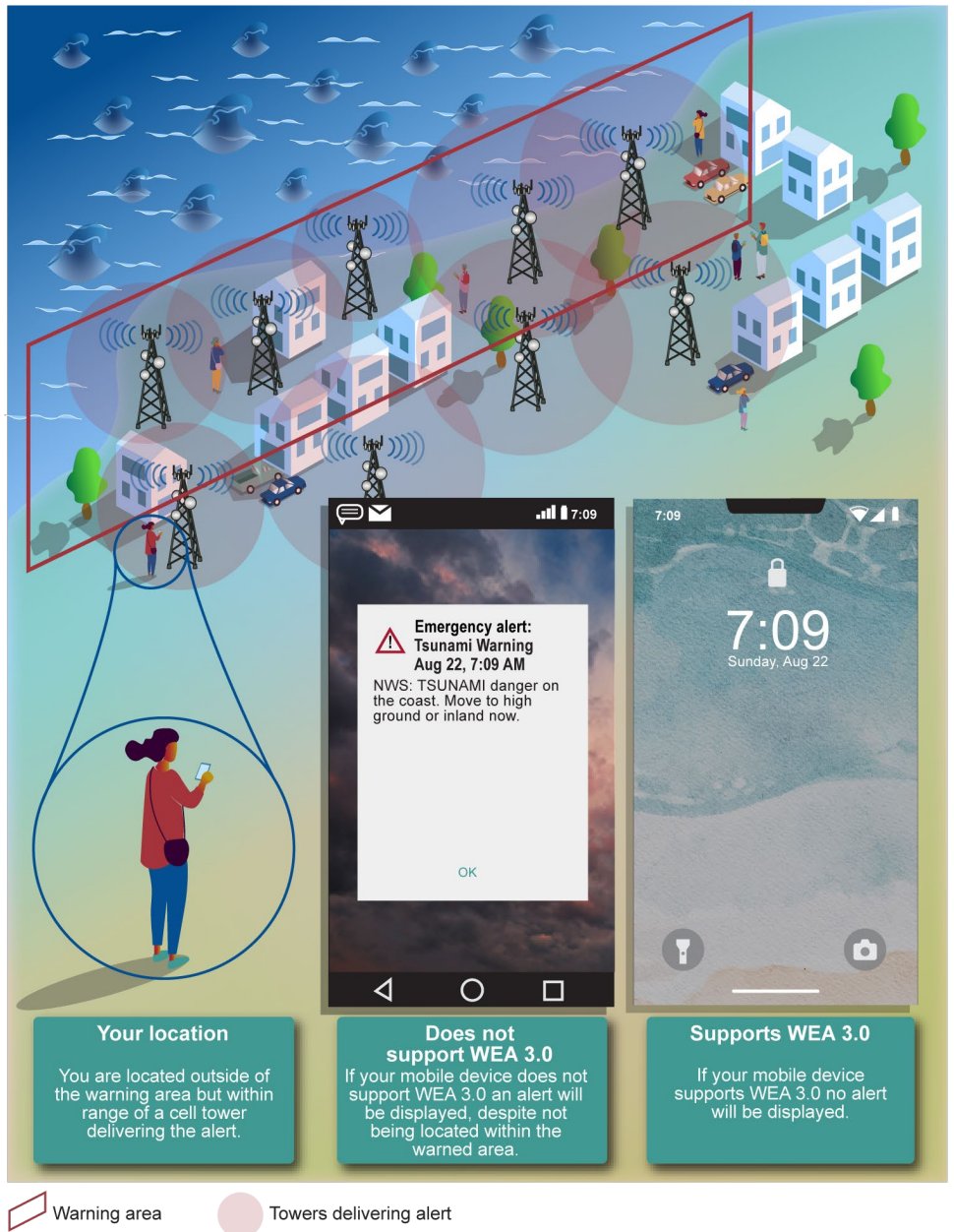
Figure 6: Wireless Emergency Alerts May Reach Some Mobile Devices Outside the Tsunami Threat Area
