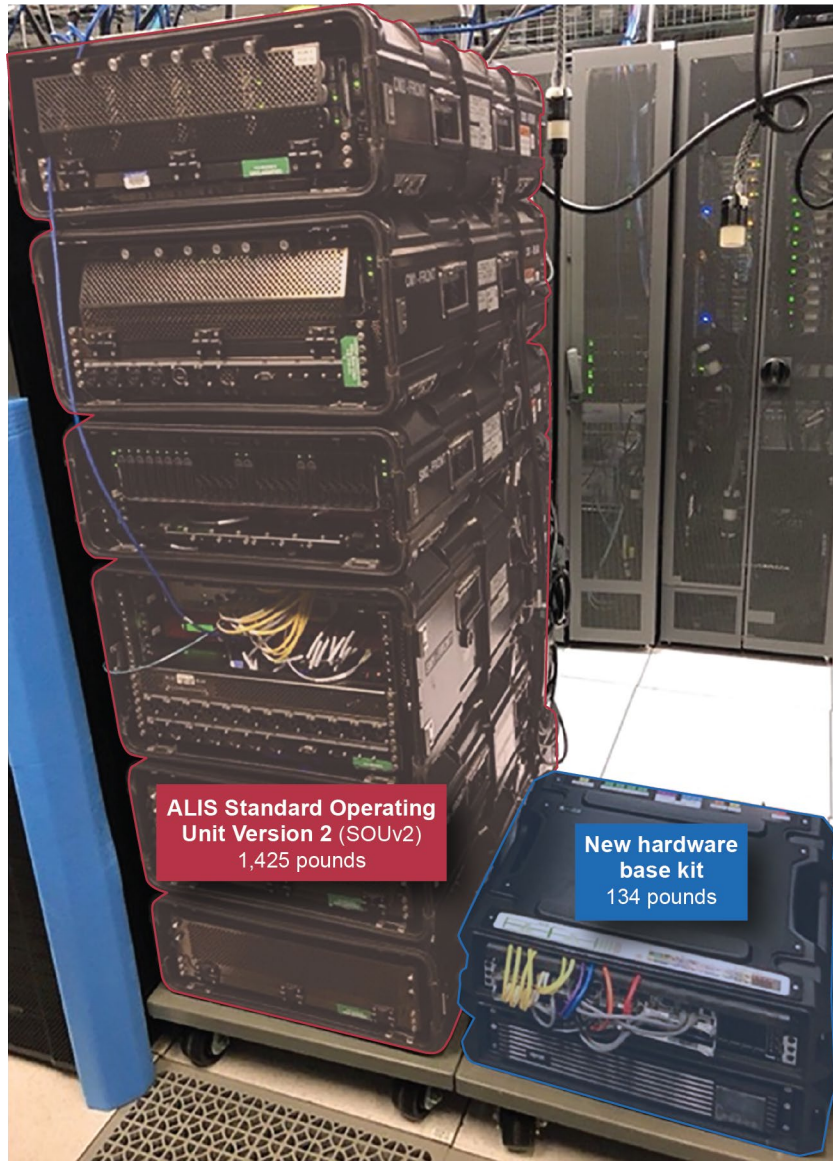
Figure 12: New Hardware Is Smaller than ALIS Hardware
