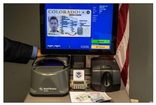
Figure 9: Transportation Security Administration (TSA) Credential Authentication Technology Machine Deployed at a Passenger Screening Checkpoint
