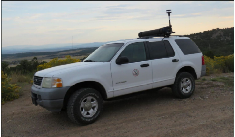
Figure 7: Methane Detection Equipment Funded with a Grant from the Environmental Protection Agency Identifies Methane Leaks from Underground Pipes
