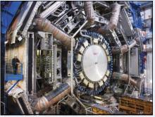
Source: © 2007 CERN. | GAO-20-268 Note: photograph above depicts the A Toroidal Large Hadron Collider Apparatus detector.
