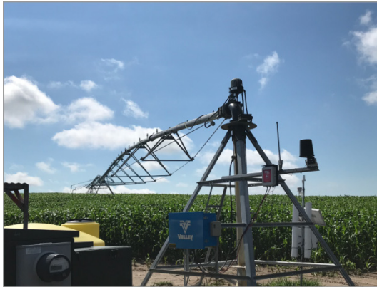
Figure 19: Example of the equipment on a center pivot that allows it to be remote controlled
