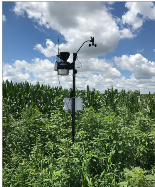
Figure 18: Wireless weather station at a farm in Nebraska
