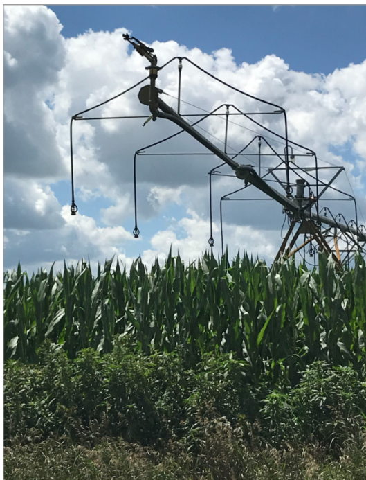
Figure 11: Another configuration of center pivot
