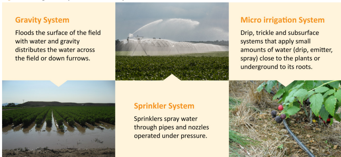
Figure 8: Irrigation systems: how they work
