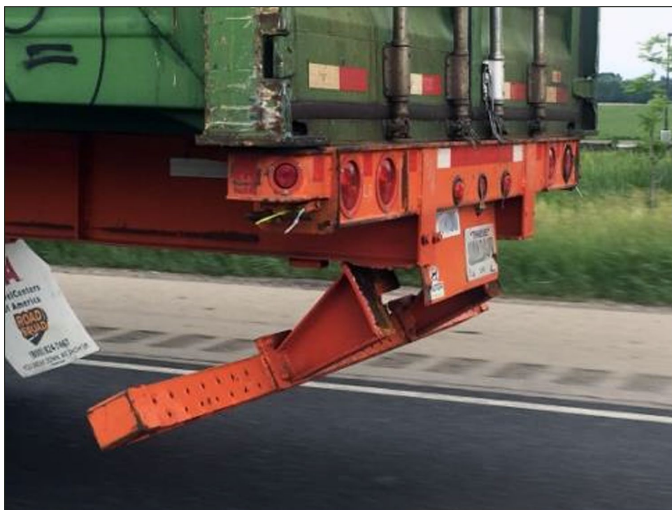
Figure 5: Example of a Damaged Rear Guard
