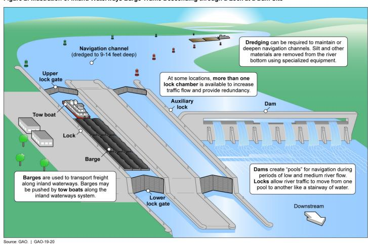
Figure 2: Illustration of Inland Waterways Barge Traffic Descending through a Lock at a Dam Site
