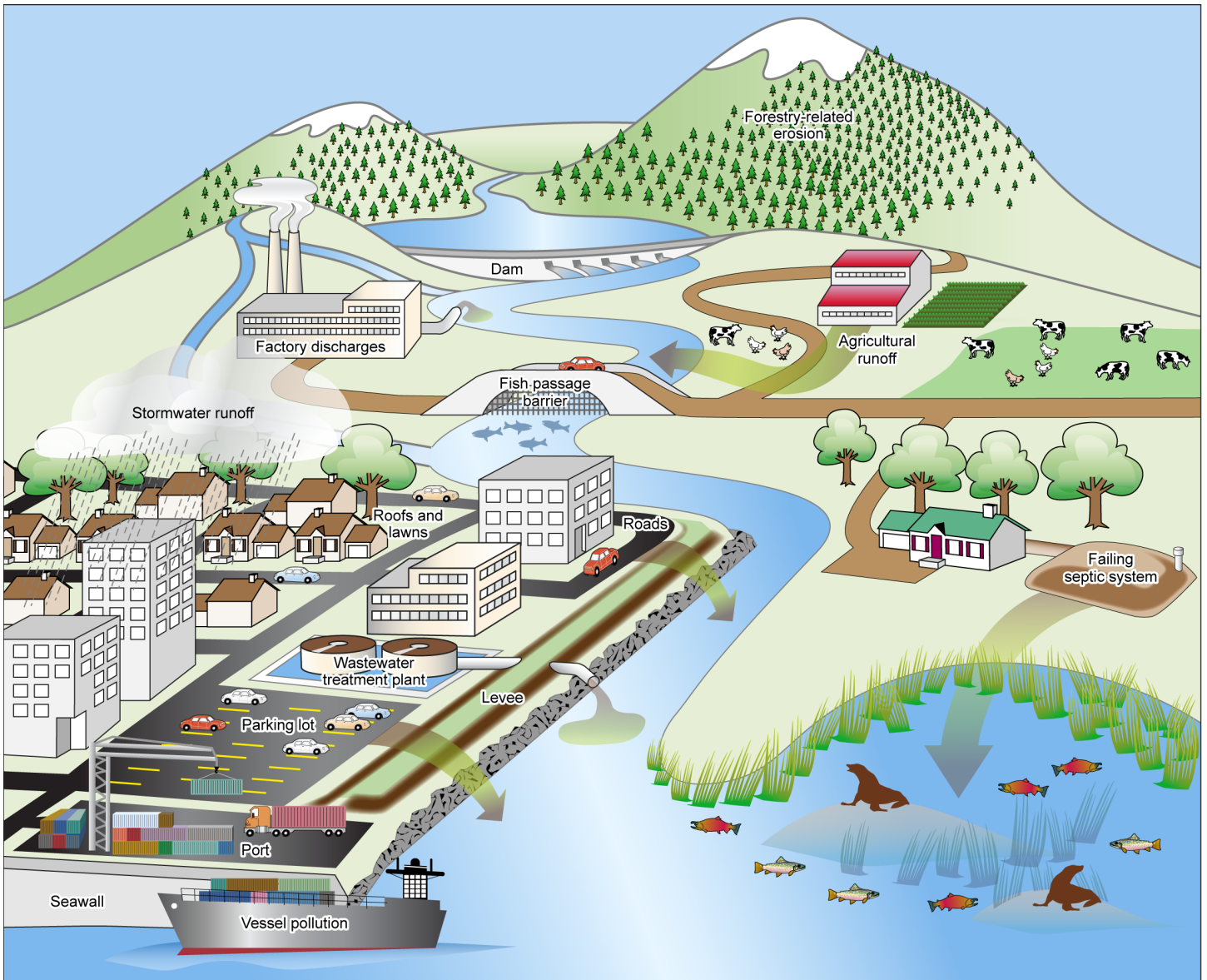
Figure 2: Point and Nonpoint Sources of Pollution That May Impair Water Quality in the Columbia River Basin
