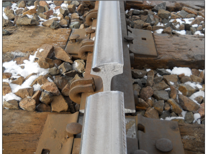
Example of excessive cold breaking a rail in half
