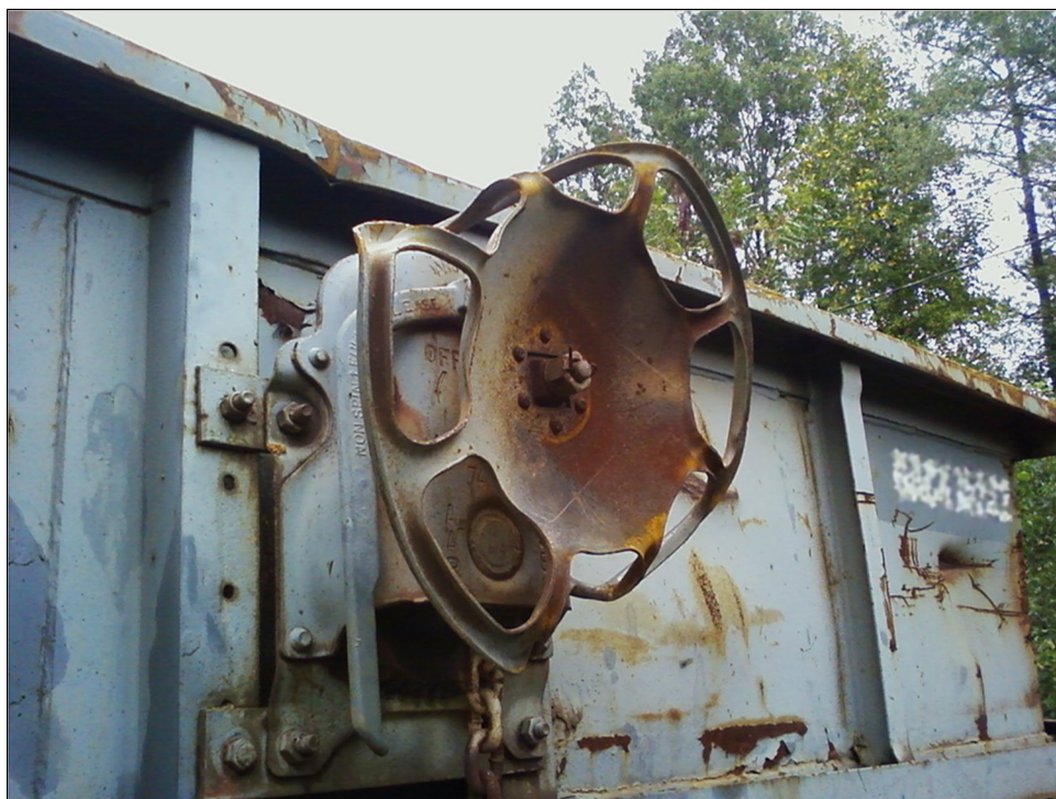
Figure 4: An Inoperable Bent Hand Brake Wheel
