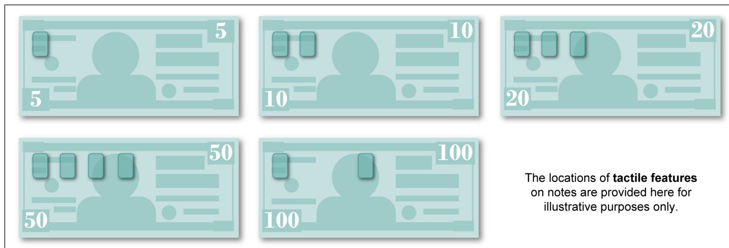
Figure 6: Raised Tactile Feature Design and Denominating Pattern Approved for Use in Testing
