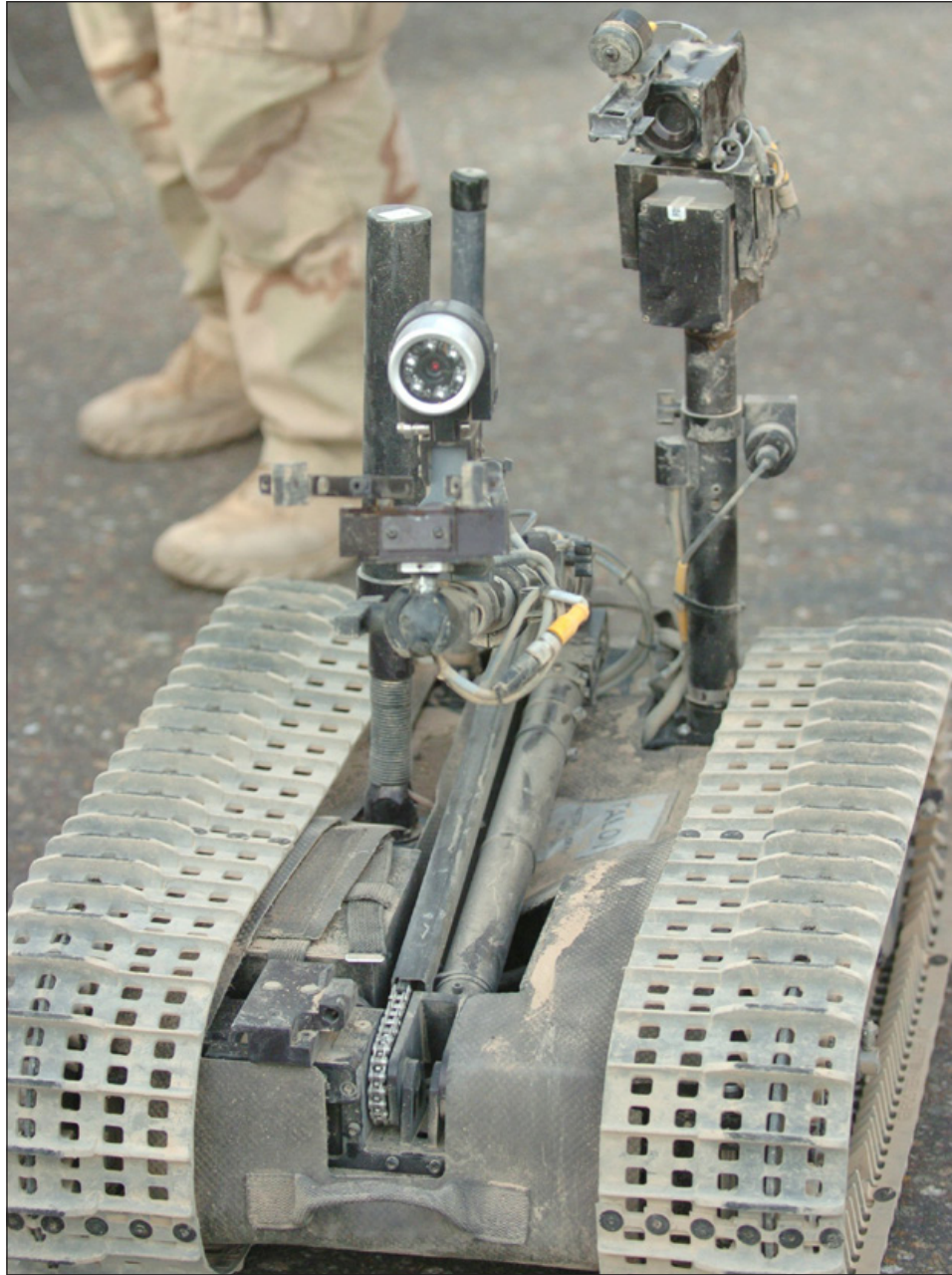
Figure 53: Remote-Controlled Robot Used by Explosive Ordnance Disposal Teams to Investigate Possible Explosive Devices Safely
