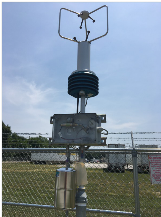
Figure 5: A sensor that triggers collection of an air sample in a canister when it detects a signal above a set threshold
