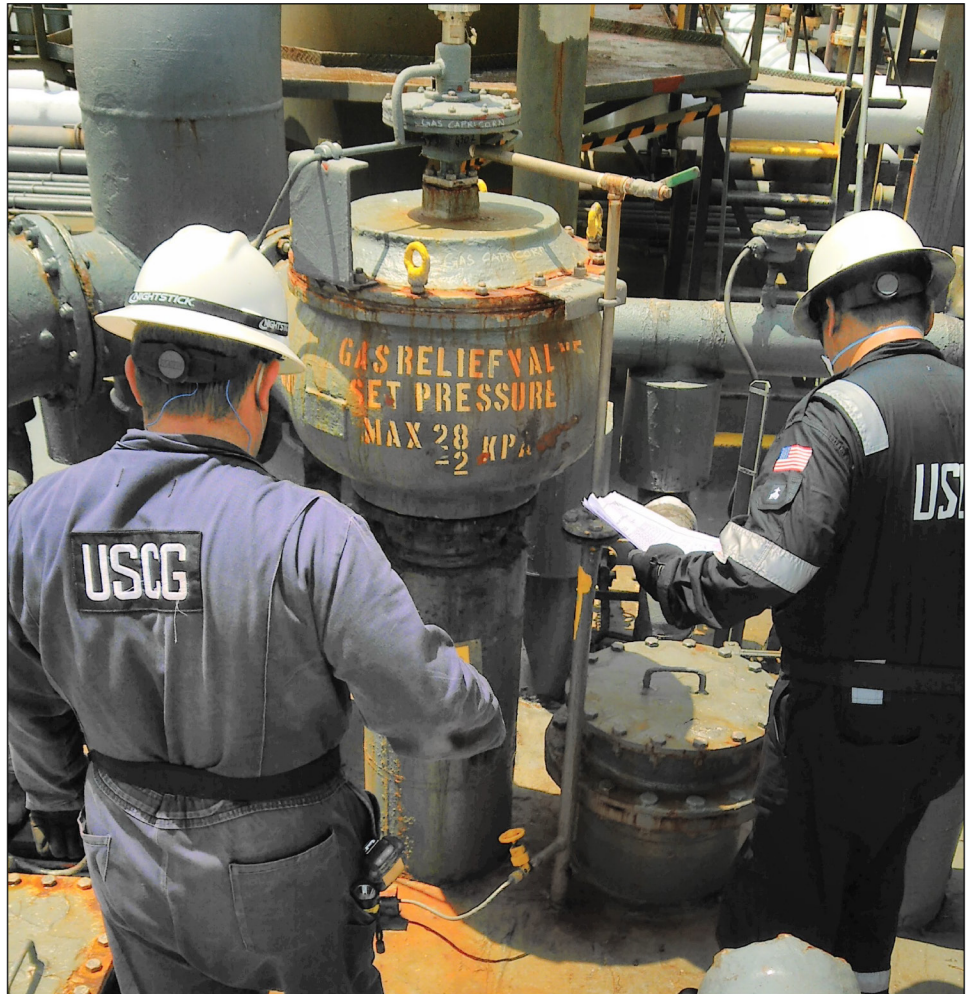
Figure 5: Coast Guard Marine Inspectors Conduct Examination of a Cargo Tank Relief Valve during a Liquefied Gas Carrier Accelerated Program Course
