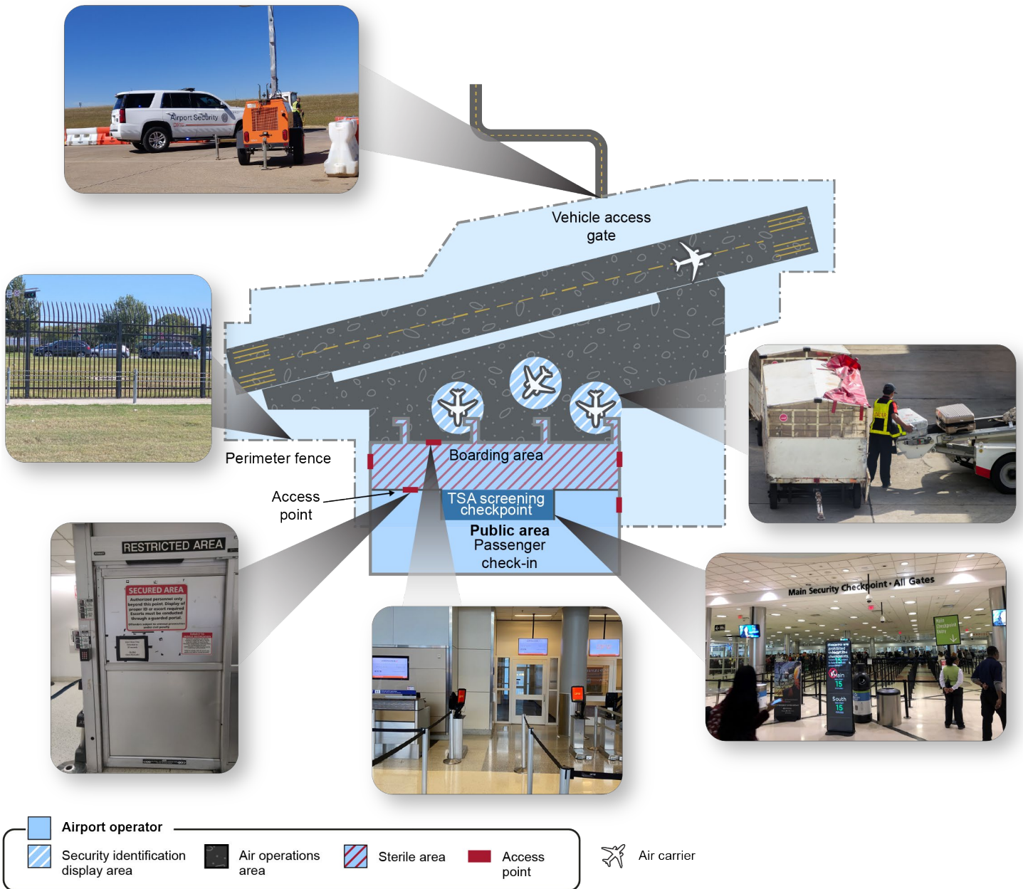
Figure 1: Illustration of Areas that May Pose Security Risks at a Commercial Airport in the United States
