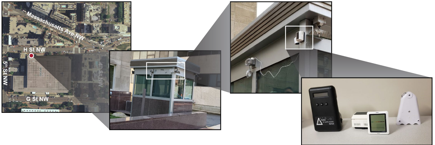
Figure 9: Low-Cost Sensors Deployed on the GAO Building
