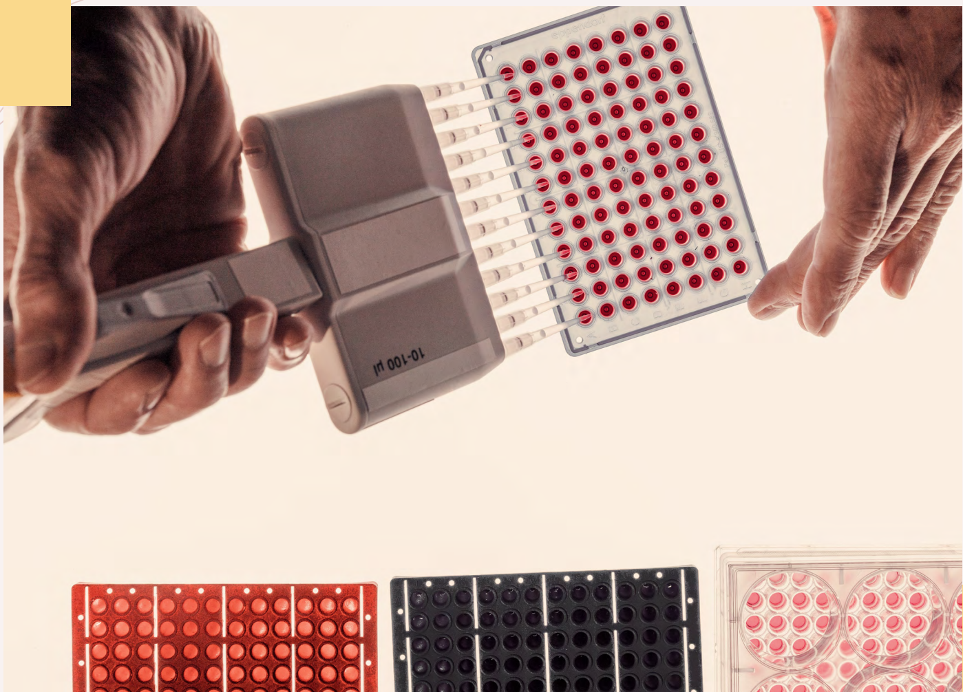
A multichannel pipette is used to prepare samples on a microplate.
