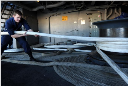
A capstan helps sailors tie the ship to the pier.
