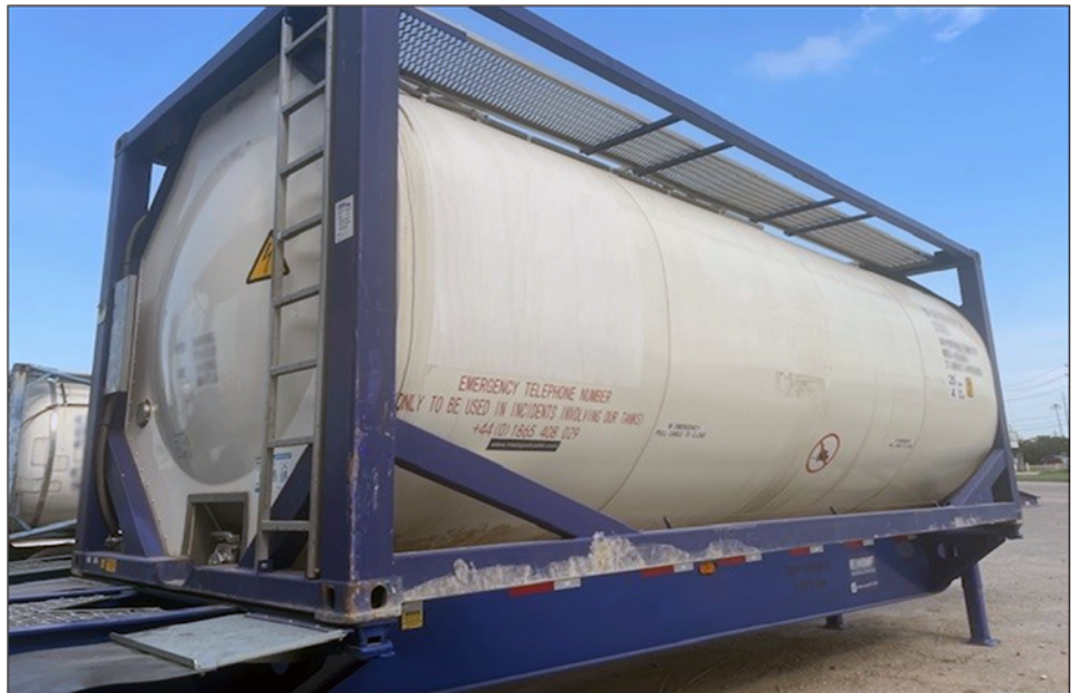
Figure 2: Cargo Container Tank Used to Transport Liquid Hazardous Materials
