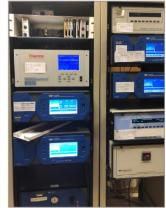
Climate-controlled shelter for reference monitoring (left) and equipment inside a reference monitoring shelter (right).
