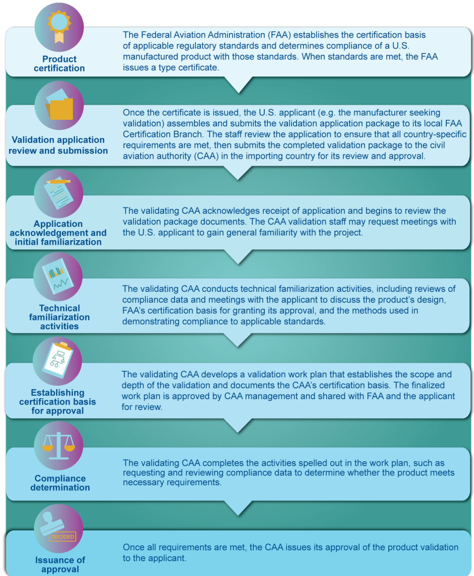
Figure 4: General Sequential Steps for Civil Aviation Authorities' Technical Validation Processes for Exported U.S. Aviation Products
