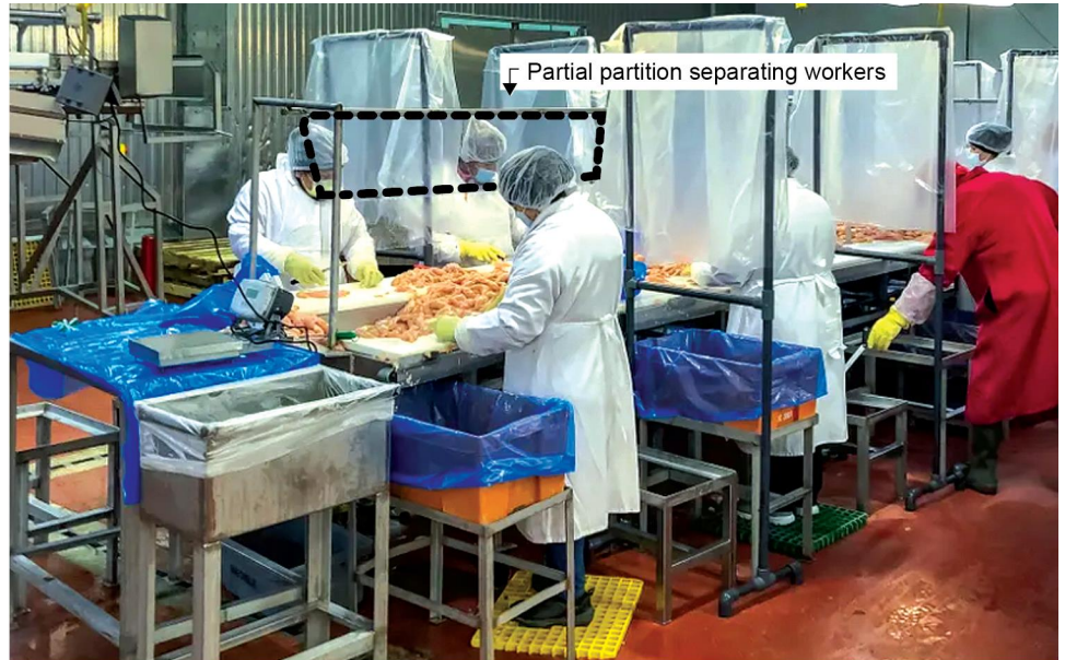
Figure 5: Plastic Sheeting between Poultry Workers and a Partial Partition Separating Workers across from Each Other
