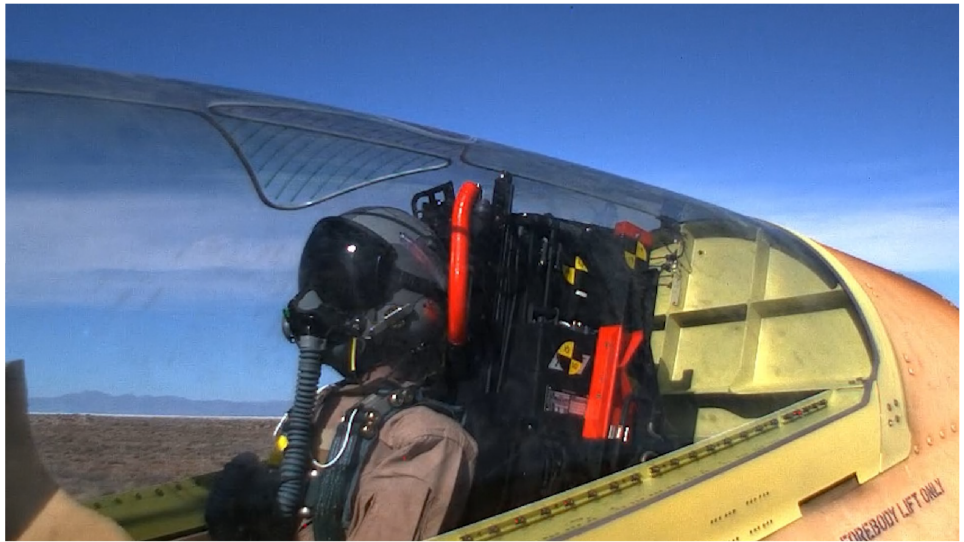
Figure 6: Advanced Pilot Trainer Ejection Seat and Canopy Fracturing System Blast Cord
