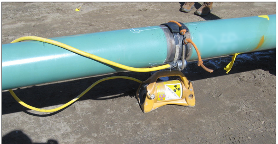
Figure 3: Industrial Radiography Device Using Iridium-192
