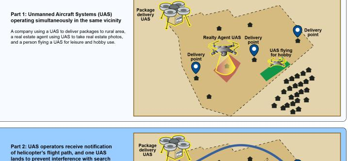
Service Suppliers. UAS operators receive notification of helicopter's flight path, and one UAS lands to prevent interference with search and rescue operation.
