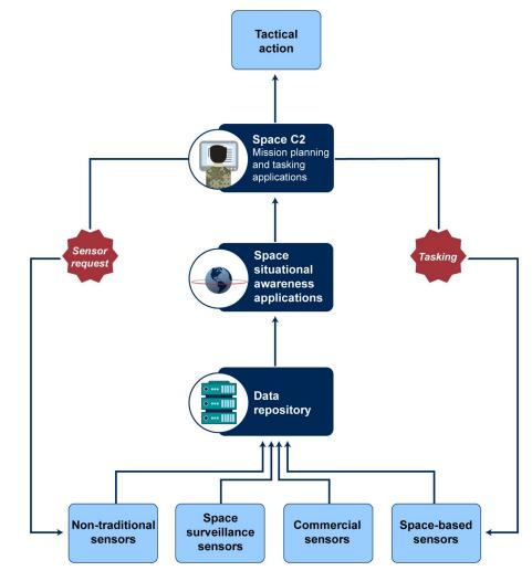
Figure 2: Space Command and Control (C2) Program Planned Construct
