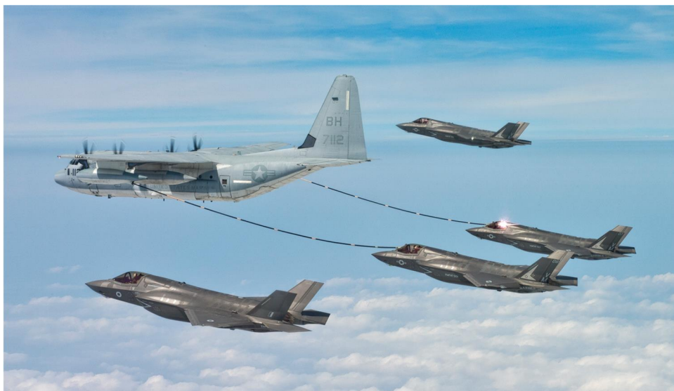
Figure 8: F-35B Aircraft Refuel from a KC-30 Aerial Refueling Tanker Using Hose and Drogue Refueling Equipment
