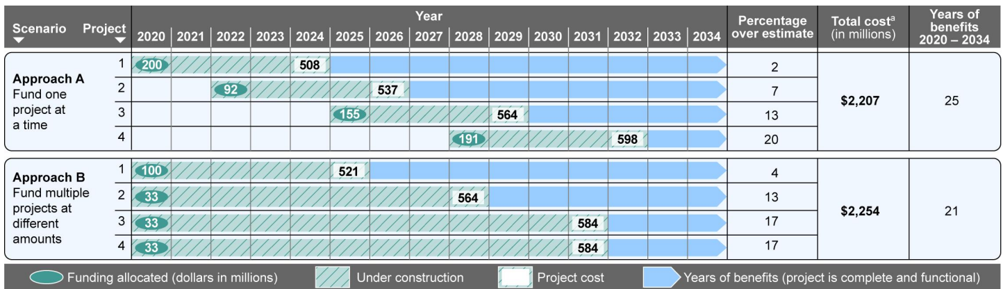
Figure 12: Comparison of Hypothetical New Construction Project Costs, Time Frames, and Years of Benefits for Two Different Funding Approaches over a 15-Year Period
