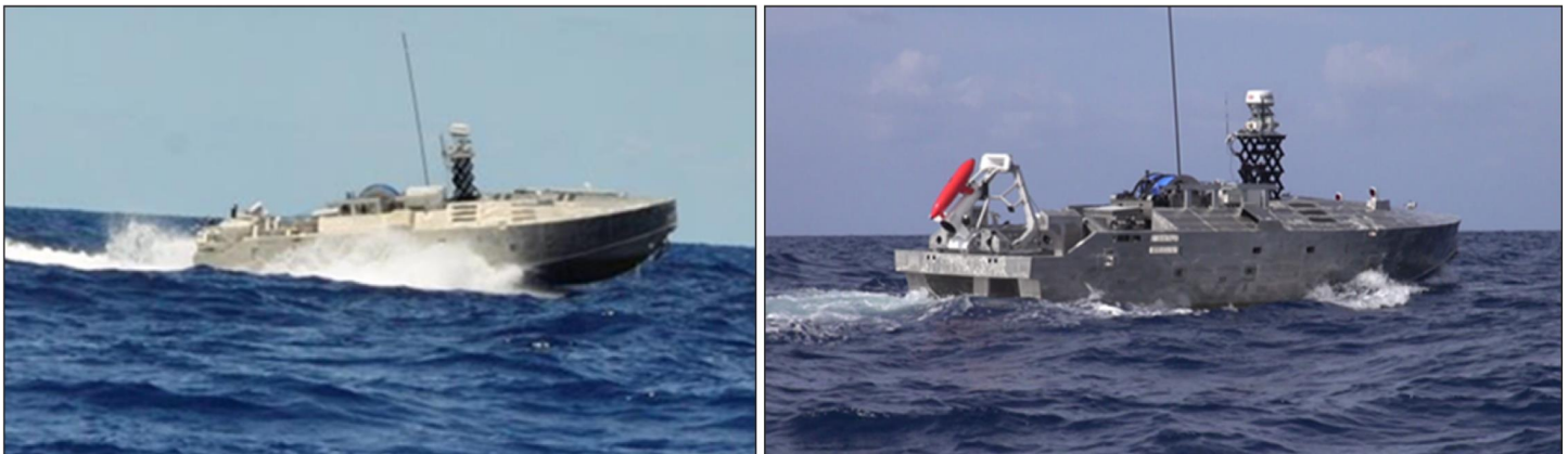
Figure 8: The Navy's Mine Countermeasures Unmanned Surface Vehicle and Unmanned Influence Sweep System
