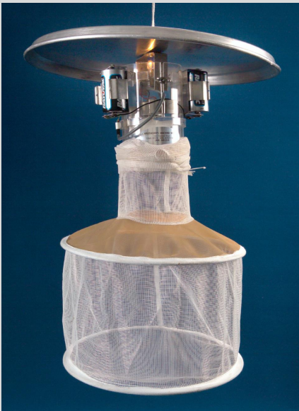
Example Mosquito Trap Used to Trap Vectors to Be Tested for Pathogens
