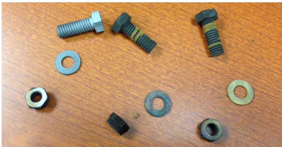
Figure 2: Army Nuts and Bolts Additively Manufactured
