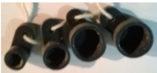
Figure 7: Tobyhanna Army Depot Dust Caps for Radios Additively Manufactured
