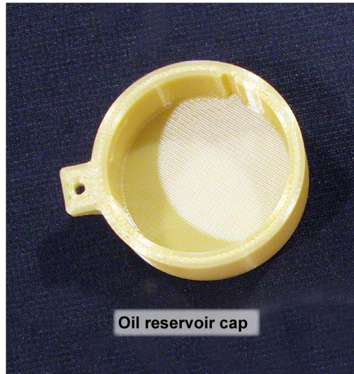
Figure 9: Navy Oil Reservoir Cap Additively Manufactured
