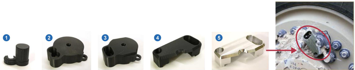
Figure 5: Army Valve Stem Cover Additively Manufactured for Interim Solution
